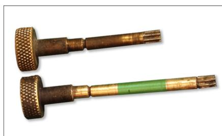
Shown is the modification of the focus knob. At the top is an original 4x5 pre-Anniversary model and at the bottom an original Top Handle 4x5 model. Shown in green are the parts brazed and turned.
