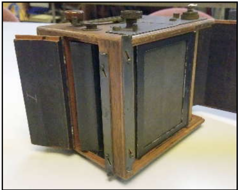
Left to right, model B prototype, prototype open, and actual production camera. It appears that film loading was simplified by removing the corner post.
