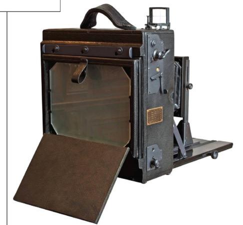
I used the old bellows as a template for a new bellows. I use a synthetic leather from DALBE [www.dalbe.fr](http://www.dalbe.fr). The handle leather is also from Chapat. I use a 1909 Singer sewing machine for the heavy leather. Another good leather source is [www.cuirdeco.fr](http://www.cuirdeco.fr).
