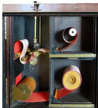
First, an overview of the film loading side with the door open and magazines with their lids removed.
