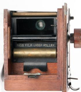
Back of camera insert, showing back of lens element reflected in mirror used to laterally correct image.
