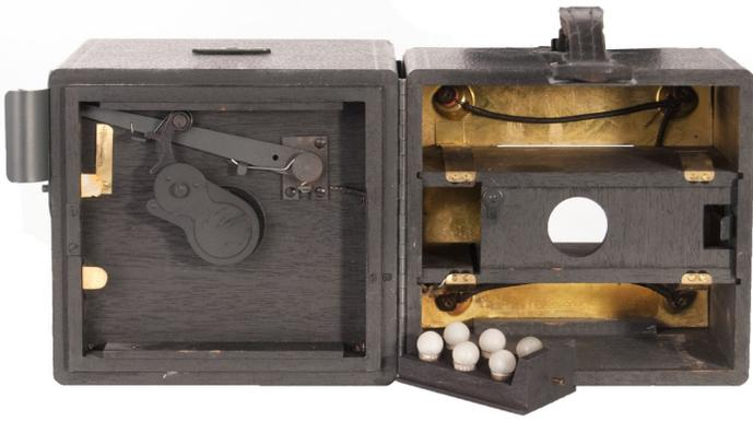
Finger Print Camera open to show built-in shutter, bulbs and battery compartments.
