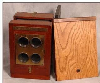
I then used a sheet of pliable plastic material with four holes to form 1/2" holes for diopters to give me an exposure of f16 that was appropriate for use with my studio strobes and Ilford FP 4 film. The strobe modeling lights provide enough light to work in without exposing the film.
