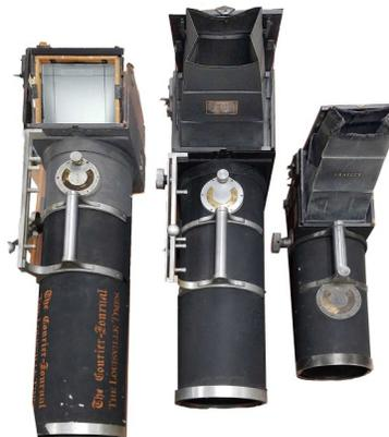
5x7 RB Graflex Series D (The hood cover is missing, so no serial #.), "Big Bertha", w/ 36-inch f/6.3 lens. Camera is marked "The Courier Journal/ The Louisville Times". Not normally made in this size.
