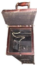
The EoP looks just like a typical floor-standing contact printer from that era. There is a handle that is raised to unlock the top cover, revealing the clear glass for receiving a contact negative and printing paper. When the handle is closed, the paper and negative are sandwiched next to the glass, and
