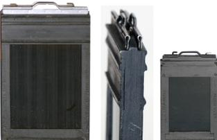
Left to right: Folmer Graflex 3 1/4x4 1/4 Type 4 Press sheet film holder (see box-end scan). Some dark slide grips are bright and some are light gray. Wood light trap covers. 2 1/4x3 1/4" Graflex Inc. Graflex-style film holder (same patent but not labeled as "Press", with metal light trap covers, and military identification numbers.
