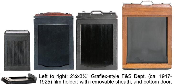
Left to right: 2 1/4x3 1/4" Graflex-style F&S Dept. (ca. 1917-1925) film holder, with removable sheath, and bottom door; two 3 1/4x4 1/4" Graflex-style F&S Dept and Folmer Graflex Corp. (1926-1944) plate holders, with removable sheaths, and fixed bottom; 4x5 Graphic-style Folmer Graflex Corp. film holder (slide removed), with fixed sheath, and bottom door.
