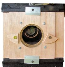
The first build did turn out okay but was a bit overbuilt regarding the screws I used. Also, the turn-locks for the scope mount were a bit underbuilt and a bit clumsy. Testing showed that I had to shim the mounting hole, so the lip of the adapter fit snugly into the hole and did not drop "off plane" under the
