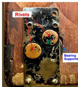
The front focus knob was repaired shoddily using a crude, hand fabricated, large rectangle brass plate, which had the original left bearing support riveted to it. It appeared to be fabricated by an 8-year-old. Underneath the large brass plate revealed a sizable countersunk hole where the original rod bearing used to reside flush against the main body.
